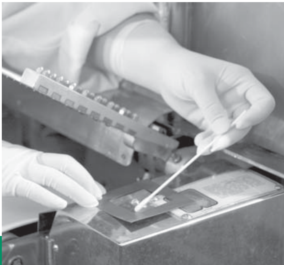
Figure 24. Smaller, tight-fitting or confined areas are best sampled for L. monocytogenes or Listeria spp. using a sterile template (2" x 2") and a moistened cotton swab.
