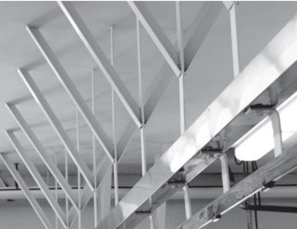
Figure 7. L. monocytogenes can travel throughout the plant in water droplets generated by the use of high-pressure hoses. Once they have found a surface to attach, L. monocytogenes can survive in dry and difficult-to-clean environments, such as overhead rails and trolleys.
