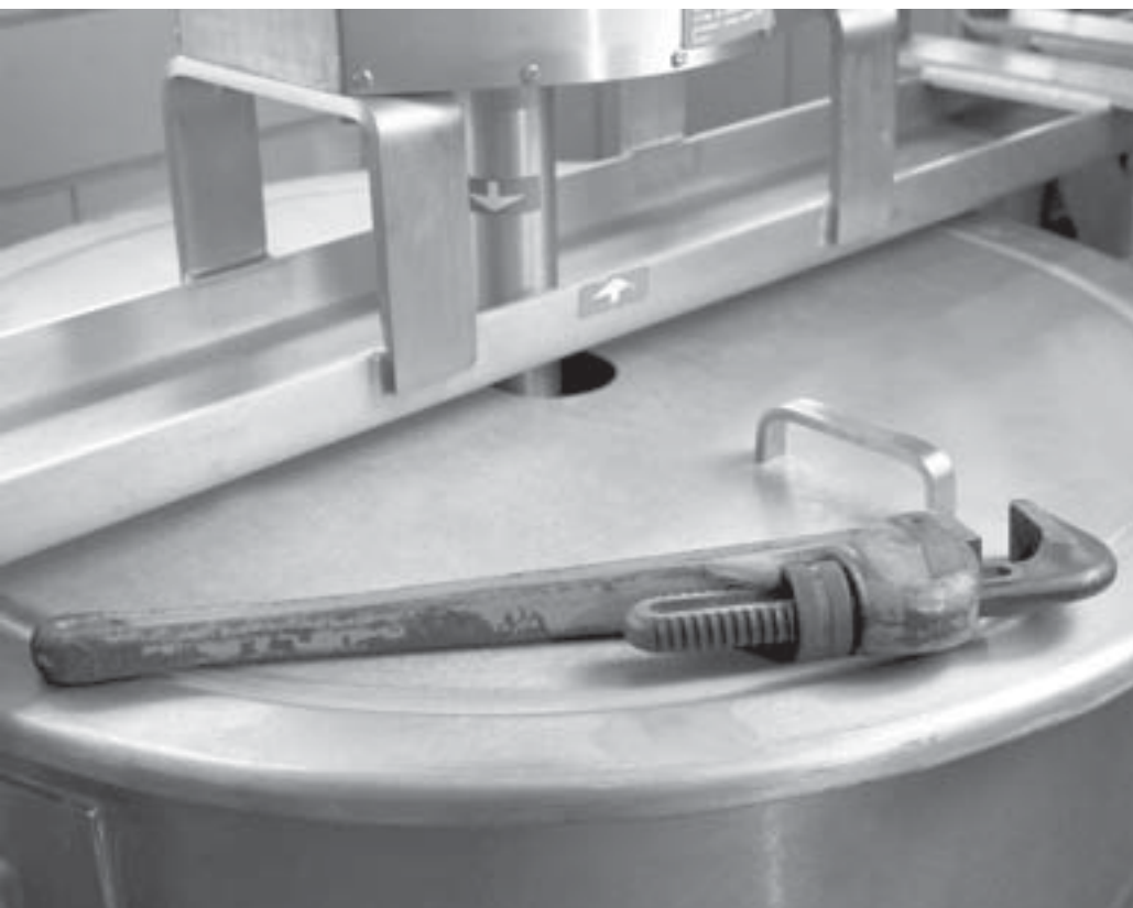
Figure 8. Maintenance tools used in raw areas may be a source of cross-contamination in ready-to-eat areas if they are not properly cleaned and sanitized prior to use.
