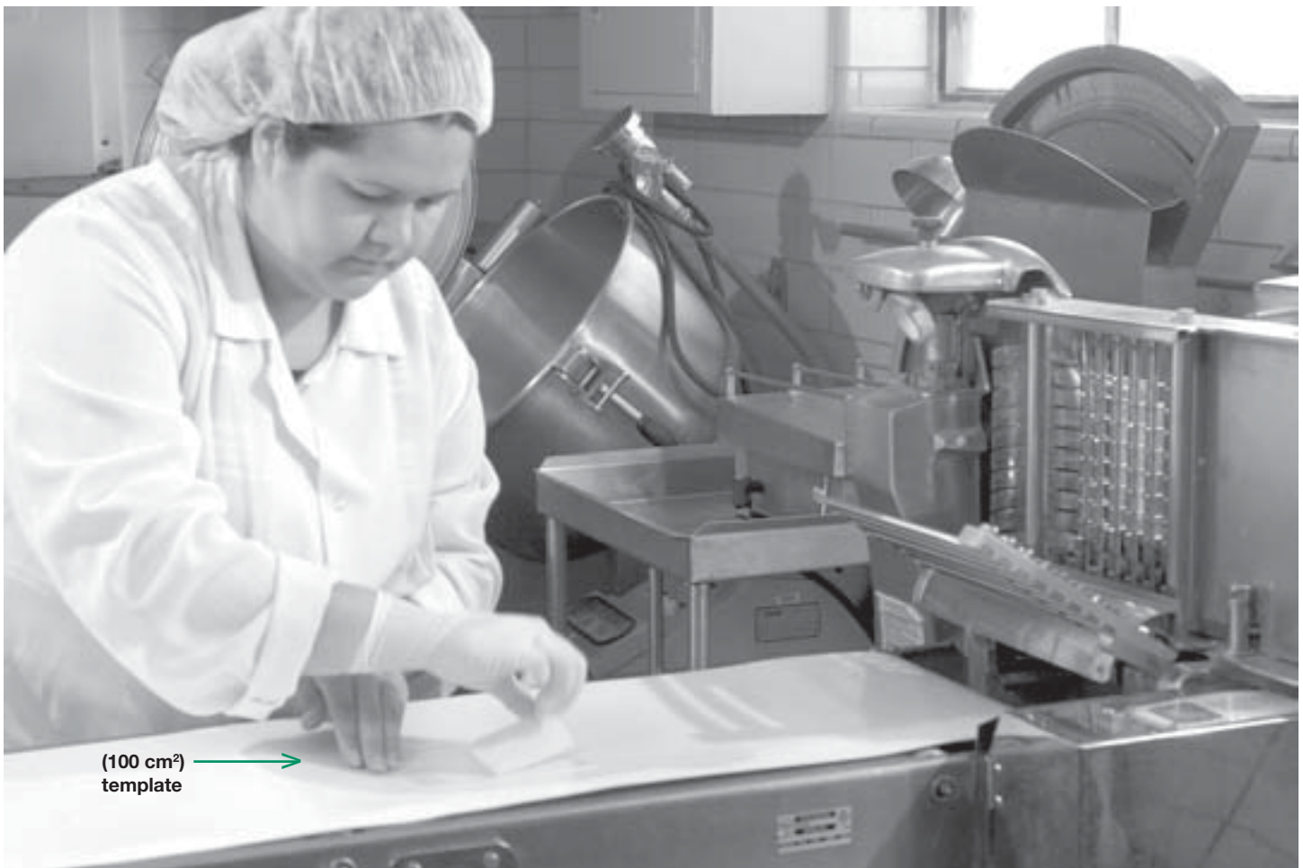
Figure 22. Large flat surfaces, such as conveyors, are best sampled for L. monocytogenes or Listeria spp. using a sterile template (10 cm x 10 cm) and a moistened sponge.
