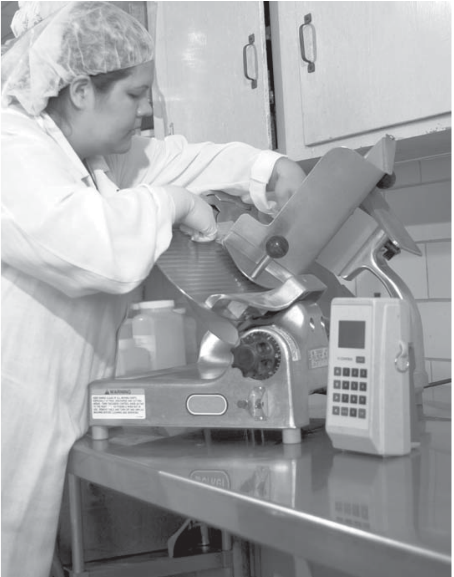
Figure 25. Machine interiors, such as deli slicers, can be assayed for ATP bioluminescence or sampled for L. monocytogenes or Listeria spp. by swabbing several sites using a moistened sponge.
