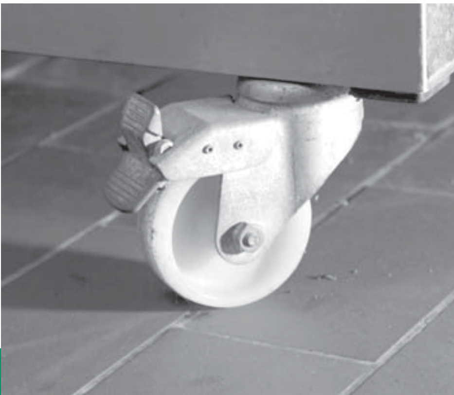
Figure 12. Wheels should be covered to prevent splash from the floor or drains. Wheels also should be easily cleaned to prevent cross-contamination of L. monocytogenes between raw and ready-to-eat areas.
