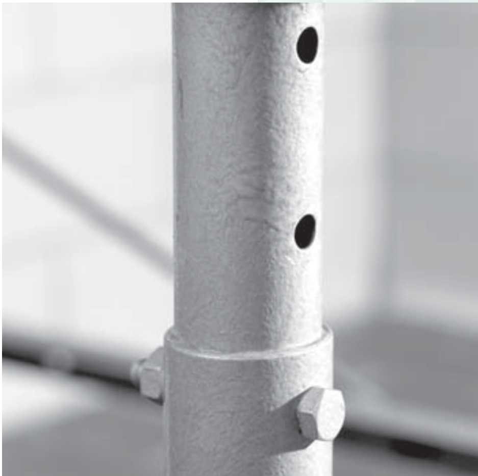
Figure 9. Hollow table legs in RTE areas may trap food and water, creating a harborage site for L. monocytogenes .
