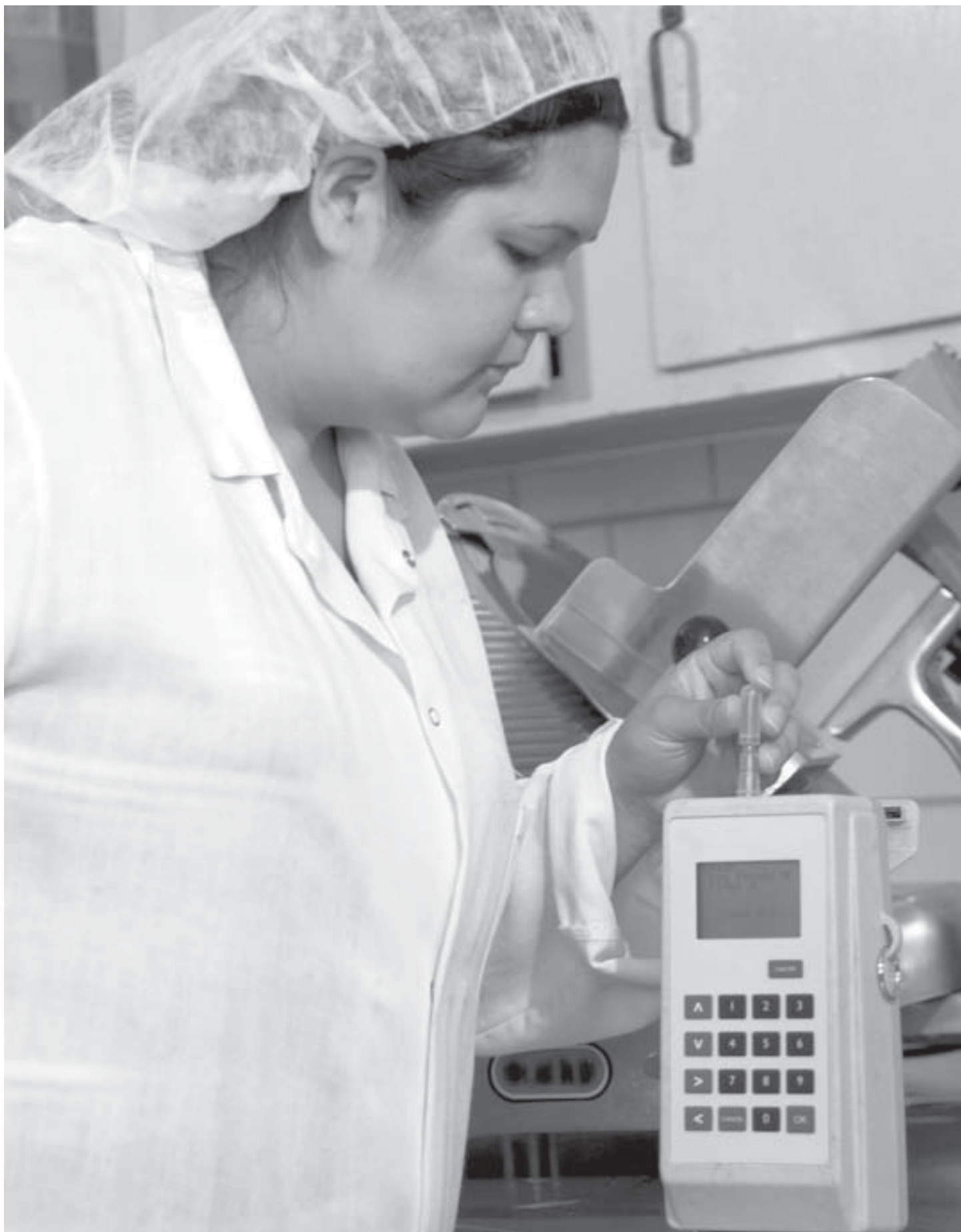
Figure 14. ATP bioluminescence systems are real-time tools that can be used to assess information about sanitation procedures.
