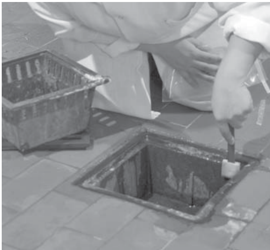
Figure 23. In order to swab drains adequately for L. monocytogenes or Listeria spp., remove drain covers and swab the interior surfaces and throats of the drain with a moistened sponge.
