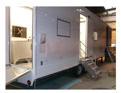
Pull out ramp to aid with getting crated birds into the bleed area- there is also a rollout awning to help protect the crated birds from inclement weather
